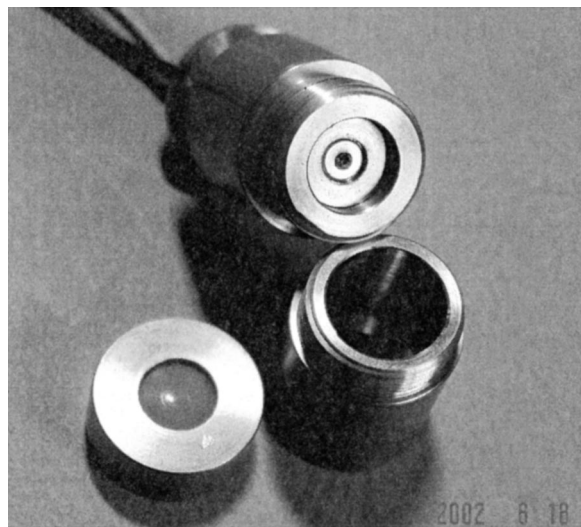
FIG. 6. A photograph of the optical structure made of copper that includes a lens and a PIR sensor set.
